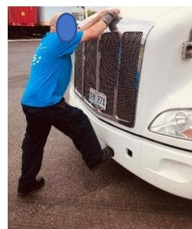
*Maintain three-points of contact to open the hood, with one foot on the ground.*
